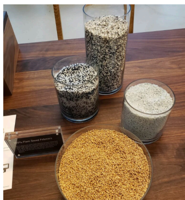
The resin pellets used to create the 3D-printed pieces is made from leftover food waste.
